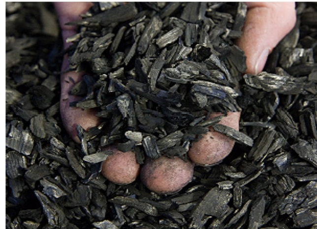
Biochar, shown above, is made from excess organic forest material and is proving to be a valuable economical and environmental resource. Photo by Pam Voth Photography.
